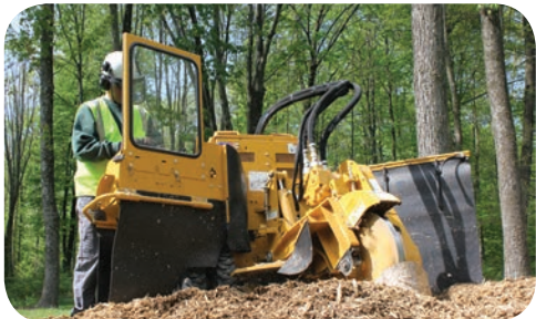
Hydrostatic Cutter Wheel Drive with "Quick-Stop"
