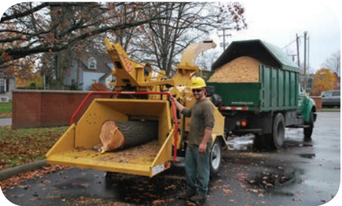
Large Feed Table with 18-inch x 24-inch Infeed Opening
