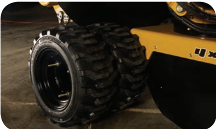
Dual Rear Wheels for Increased Stability and Traction
