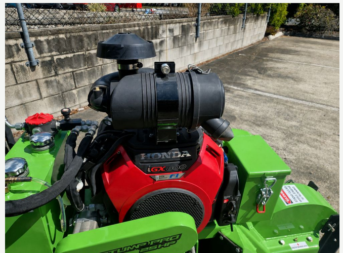
Engine bay — Donaldson air filtration
