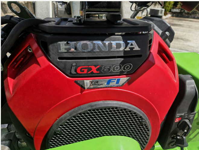
Honda iGX800 — fuel-injected V-twin
