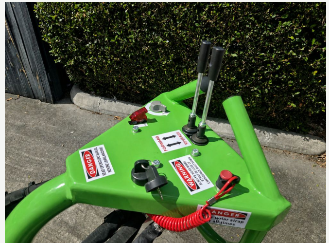
Controls — forward / reverse and kill switch
